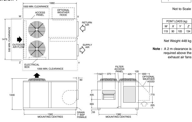
Fig. 2 Downward Supply Air / Mounting Rails Version 2
