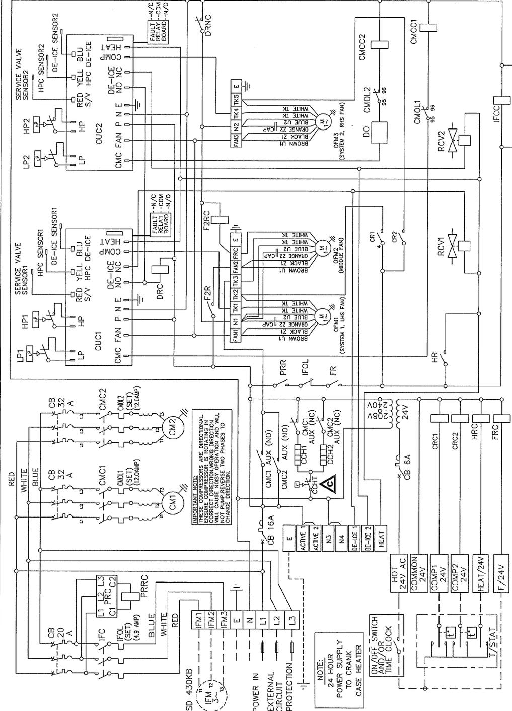
NOTE: CONTROL TRANSFORMER 240V PRIMARY VOLTAGE IS USED FOR COUNTRIES WITH 230 - 240V POWER SUPPLY. FOR COUNTRIES WITH SUPPLY VOLTAGE 200 - 220V CHANGE PRIMARY VOLTAGE TO 208V ON TRANSFORMER.
