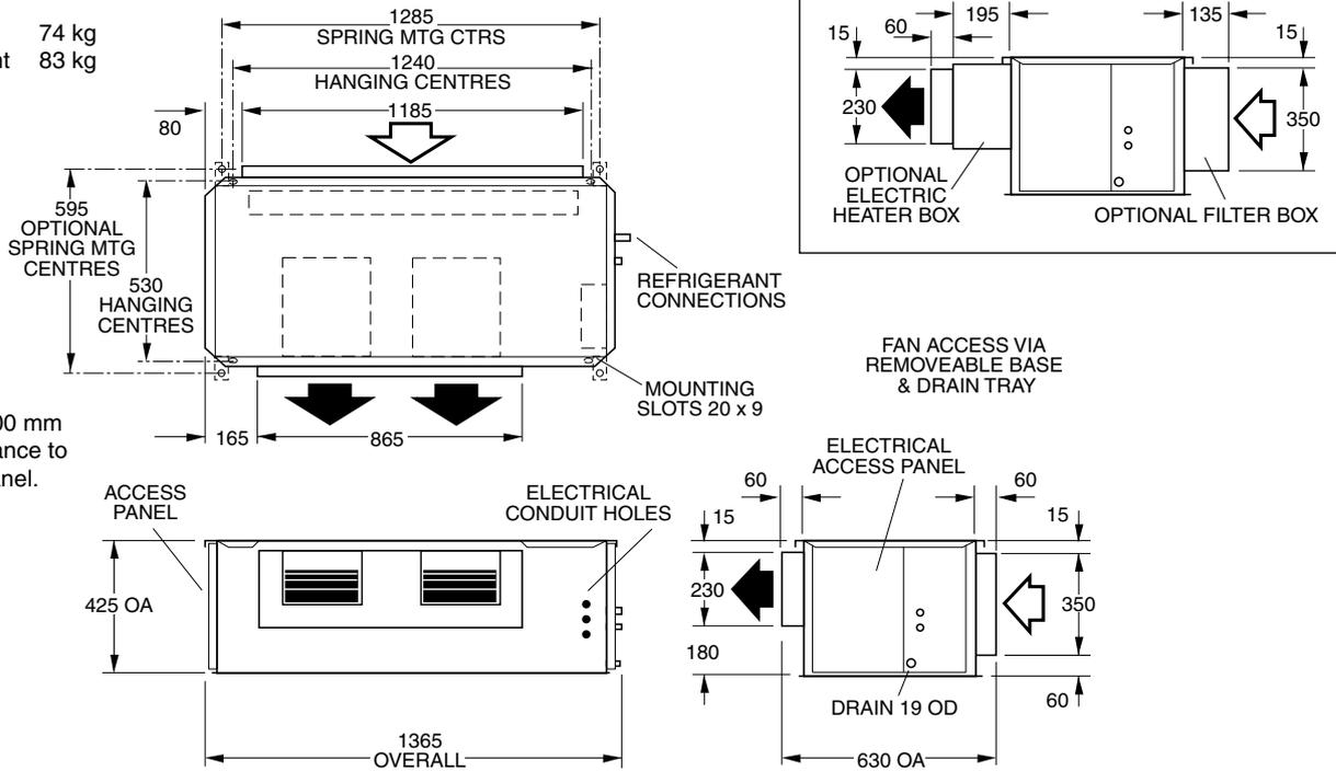
**Note :** Allow 500 mm minimum clearance to each access panel.
