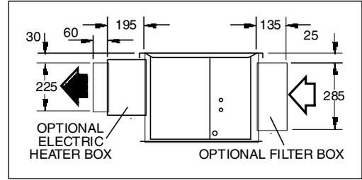
FAN ACCESS VIA REMOVEABLE BASE & DRAIN TRAY
