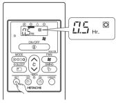
Operation will start for setting temperature at setting timer (The starting time may different depend on the room temperature and set temperature).
