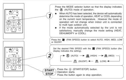
As the settings are stored in memory in the remote controller, you only have to press the ① (START/STOP) button next time.
