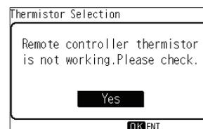
Thermistor of remote controller is not working.
