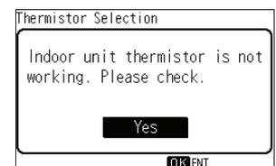
Thermistor of indoor unit is not working.
