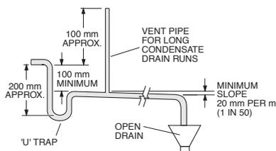
Figure 1 Condensate Drain
