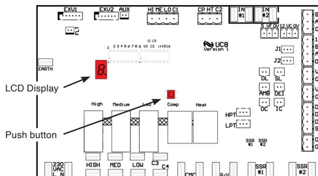
The temperzone Unit Controller 8 (UC8) is the successor to the UC6 controller. Each dual compressor OSA unit utilises two UC8 Controllers, one for each refrigeration system. The UC8 controllers receive requests such as 'Unit On/Off', 'Start compressors', 'Activate HEAT (Reverse Cycle)' and transfer the requests to the outputs after enforcing safety timers.
