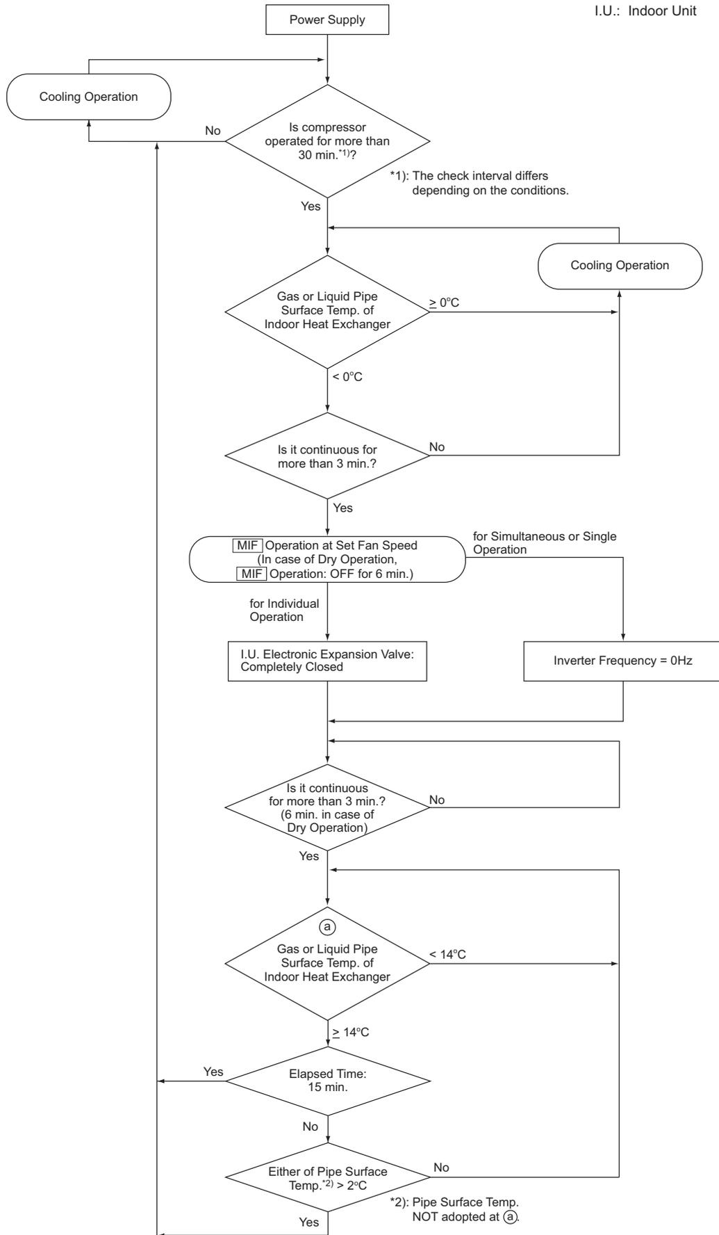
**■ Prevention Control for High Pressure Increase during Cooling Operation**
