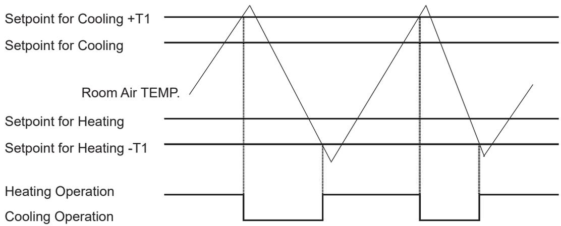
T1: Differential temperature for cooling/heating changeover
