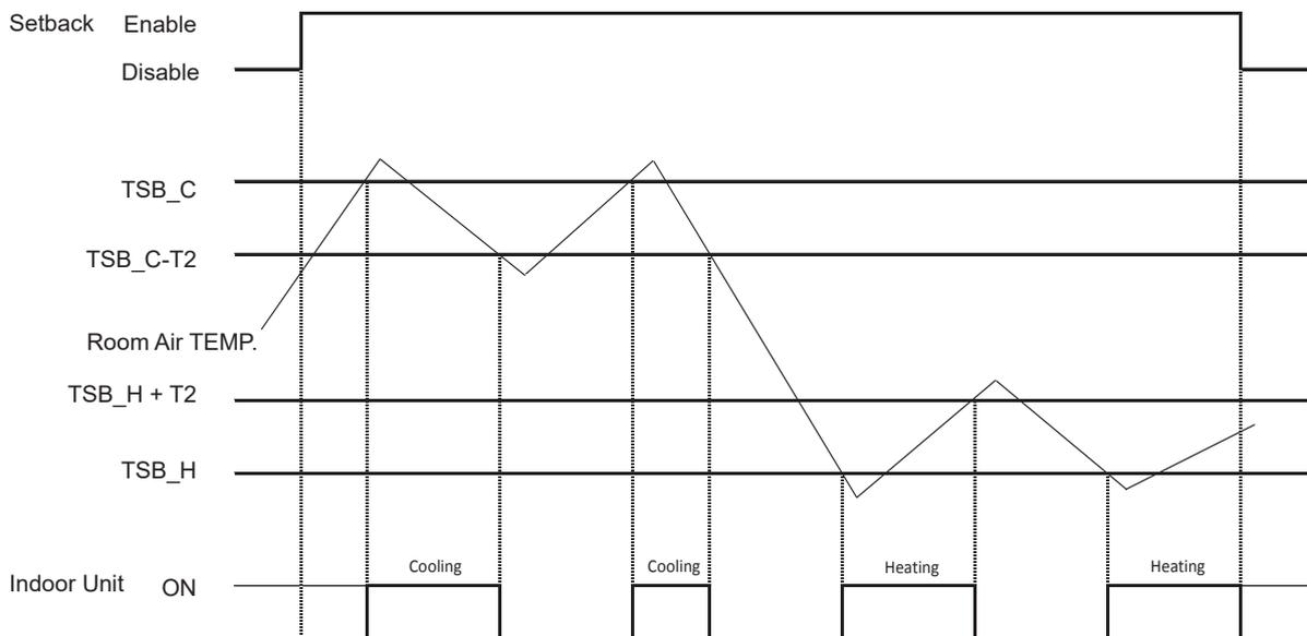
TSB\_C: Setback operation starting temperature for cooling.
