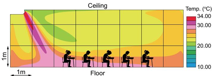
The comfortable heating air reaches every corner of the room, mainly around floor, during the heating operation.
