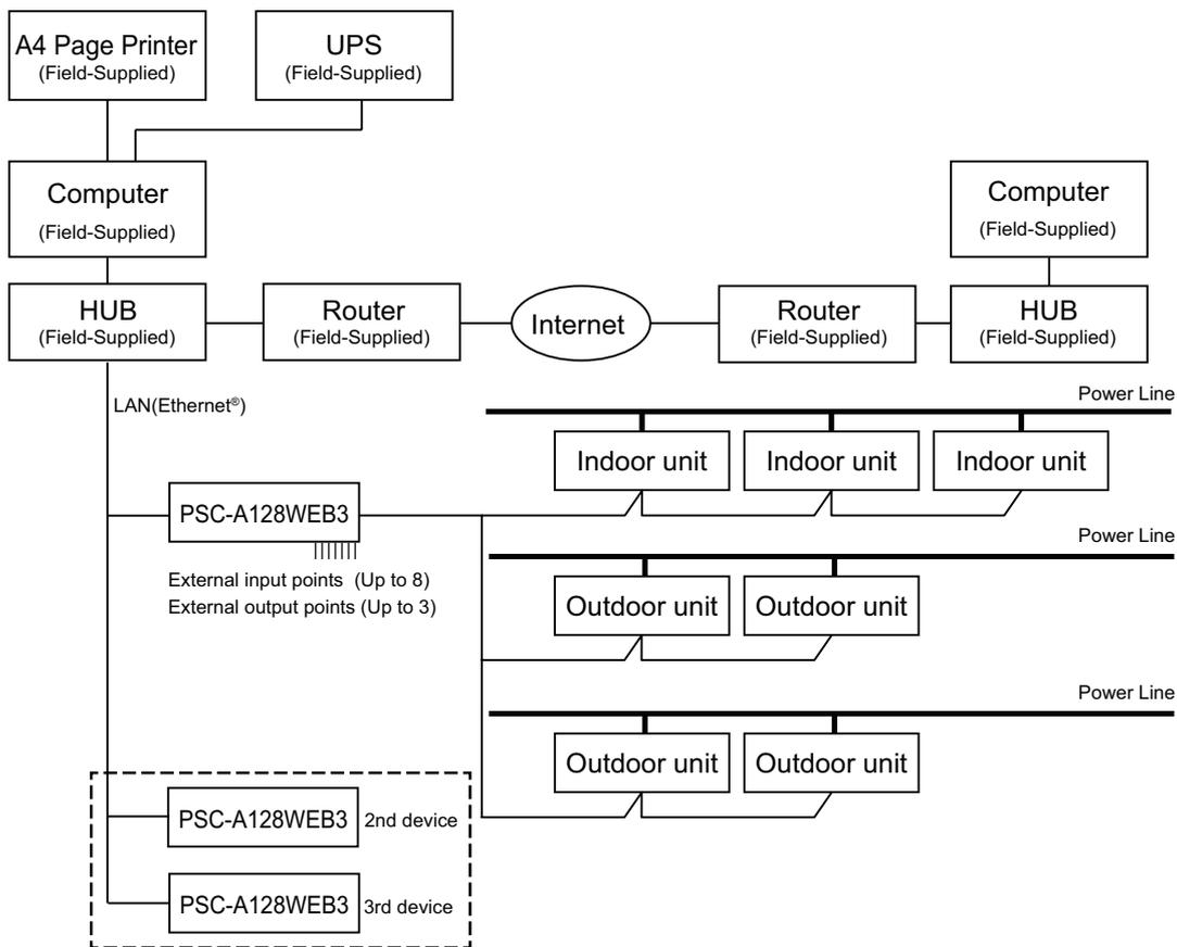
The 2nd and 3rd device connection is possible when air conditioning proportional rate division is not complete.
