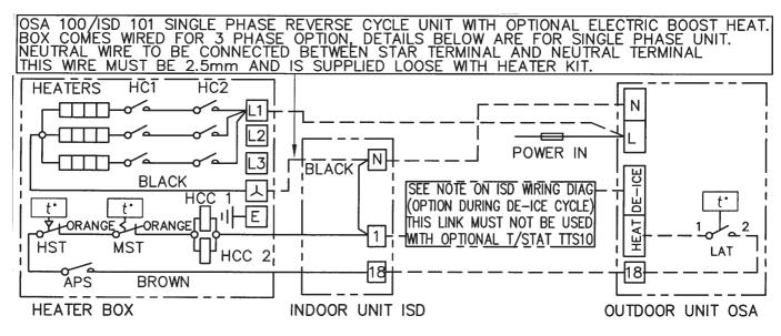
Fig. 10 3 Element, 3 Phase, Reverse Cycle Systems with Optional Electric Heat
