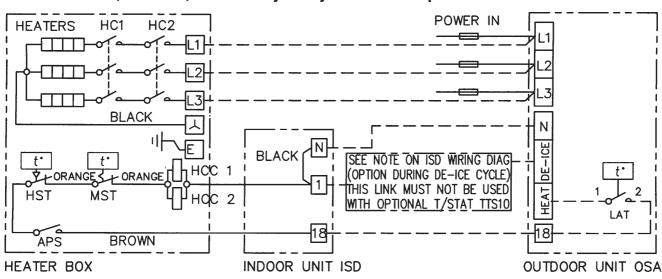
Fig. 11 3 Element, 3 Phase, Cooling Only Systems with Optional Electric Heat
