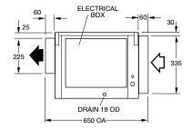
FAN ACCESS VIA REMOVEABLE BASE & DRAIN TRAY
