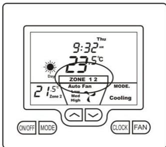
If zoning is enabled the word “Zone” and either “1”, “2,” or “1 2” (indicating both zones) will be shown. To select which zone(s) you wish to be controlled, simply tap the On/Off button to toggle between zone 1, Zone 2 or both zones
