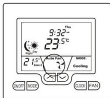
If your air conditioning system has only one Indoor fan speed, the words “High”, “Med” or “Low” will be absent from the TZT-701 Wall Control display, as shown in the picture to the left.
