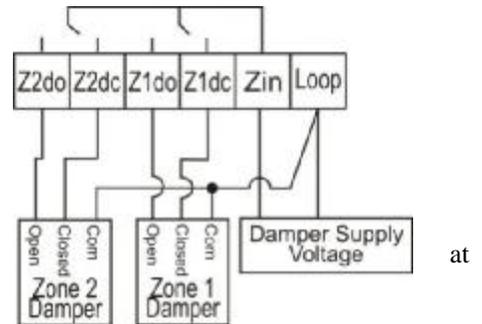
As a consequence of this advanced zone management method there may seem to be unusual delays before heating or cooling starts. The TZT-701 has time delays in place that provide adequate time for zone dampers to move to their correct position prior to starting the heating or cooling. When commissioning the zoning system patience may be required as some delays are up to 4 minutes in length to give zone dampers time to move, and for run-on delays to expire.
