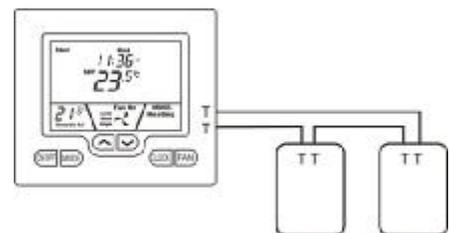
Multiple remote sensors can be used where the temperature averaging of a larger area is required. A combination of our TZT701-RS1 and TZT701-RS2 sensors may be required to satisfy complex sensor "averaging" configurations. More examples of sensors configurations are given on page 12.
