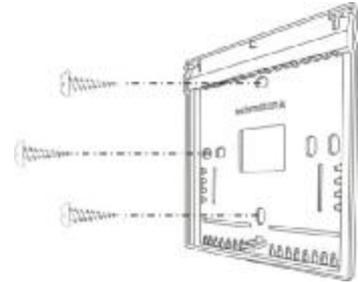
Place the "Communication Cable" and any "Remote Temperature Sensor" wires, if applicable (see the bottom section on this page), through the large opening in the thermostat base plate. Then place the thermostat base on the wall and using appropriate screws, firmly attach the base to the wall. Seal any holes where cables enter the back of the thermostat.
