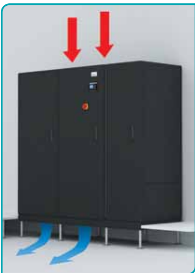
Standard version with suction from above and downflow air supply, with plinth for raised floors.
