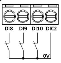
The digital input port common pins DIC1 and DIC2 are internally directly connected to the local board 0V.
