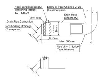
Tightening Torque: 3.0 - 3.5N.m
