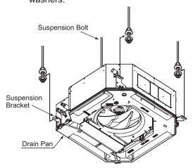
Fig. 4.7 Mounting the Indoor Unit
