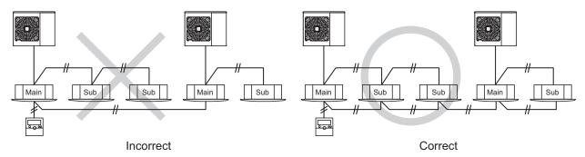
(b) Connection between Main Unit without Transition Wiring and Unit with Transition Wiring When the indoor units in multiple refrigerant cycles are controlled by one remote control switch, all the indoor units are required to be connected with the transition wirings.
