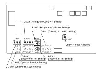
(4) Capacity Code Setting (DSW3) No setting is required, due to setting before shipment. This switch is utilized for setting the capacity code which corresponds to the Horse Power of the indoor unit.
