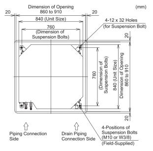
Fig. 4.3 Opening of False Ceiling and Suspension Bolts
