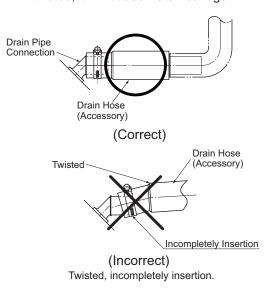
Fig. 6.2 Insertion of Drain Hose
