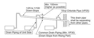
(e) The drain hose must be performed with a horizontal or upper-slope to prevent the airpocket inner the drain hose. If the airpocket occurs, the drain water will flow back to the unit and the abnormal noise and leakage to the room will occur when the unit operation is stopped.
