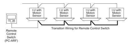
(3) In the case that 2 remote control switches are connected, the motion sensor can be set on only the main remote control switch. The sub remote control switch is for the indication only.
