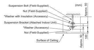
Fig. 4.6 Mounting Nuts and Washers
