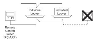
(4) The individual louver function is not for blocking the air outlet. If the air outlet is blocked, 3-Way Outlet Parts Set shall be used.
