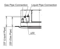
Fig. 5.1 Position of Piping Connection
