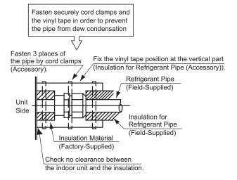
Fig. 5.3 Insulation on Pipes
