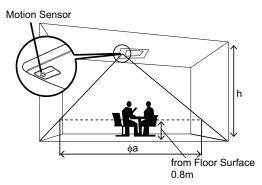
Consider the air distribution from the indoor unit to the space of the room, and select a suitable location so that uniform air temperature in the room can be obtained.
