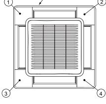
(b) Remove the electrical box and connect the relay wire (attached in the air panel) to CN10 in the electrical box as the following figure.
