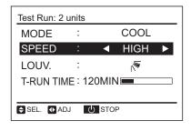
(c) Press "△" or "¬", select "LOUV." and select " " (auto swing) by pressing "¬" or "¬". The auto swing operation will be started. Check the operating sound at the louvers. If abnormal sound is generated from louvers, it may be a deformation of the air panel due to incorrect installing. In this case, install the air panel again without a deformation. If abnormal sound is not generated, press "¬" or "¬" again to stop the auto swing operation.
