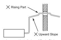
Incorrect Installation of Drain Piping
