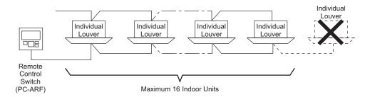
(2) The individual louver setting in the same refrigerant cycle are available up to 4 indoor units without the transition wiring for the remote control switch.
