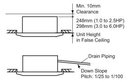
Fig. 4.2 Installation Location of Indoor Unit
