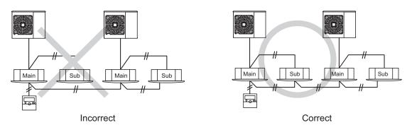
(c) Connecting Remote Control Switch to Sub unit without Transition Wiring When the indoor units are controlled by 2 remote control switches, the sub remote control switch shall be connected to the main unit.
