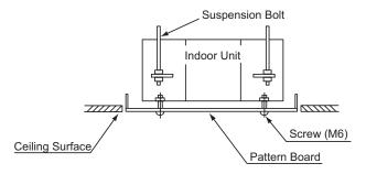
(3) Tighten the nuts of the suspension brackets after the adjustment is completed. Apply LOCK-TIGHT paint to the bolts and nuts in order to prevent them from loosening. When adjusting the space between the indoor unit and the ceiling surface, maintain the levelness of the indoor unit. If the levelness is not maintained, it may cause a malfunction of the float switch.
