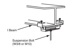
Fig. 4.4 Mounting the Suspension Bolts
