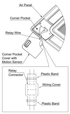
(d) Catch the band at the rear side of the corner pocket cover with motion sensor onto the projection at the air panel as shown in the figure below.
