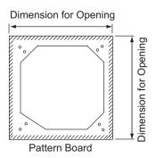
(d) Ceiling Not Completed with Panels yet When the false ceiling is not completed yet, attach the pattern board to the indoor unit with the screw (M6), as shown in the figure. And specify the location of the opening. Adjust the position of the indoor unit as the procedure (b) after ceiling is completed with the panel.
