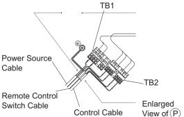
Fig. 7.1 Electrical Wiring Connection for Indoor Unit
