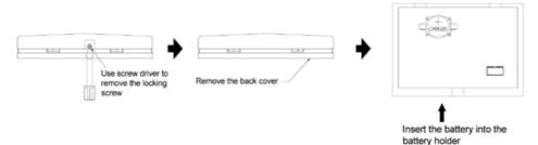
Remove and replace the battery with a lithium CR1220 cell battery.
