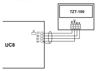
Note: Capacity Staging. A TZT-100 must be configured for single-stage operation, the default setting.
