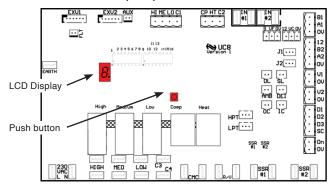
The UC8 controller receives requests such as 'Unit On/Off', 'Start compressors', 'Activate HEAT (Reverse Cycle)' and transfer the requests to the outputs after enforcing safety timers.
