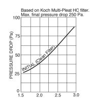
If using EU-2 filter media, provide 0.08 m<sup>2</sup> face area per 100 l/s of airflow to maximise efficiency.
