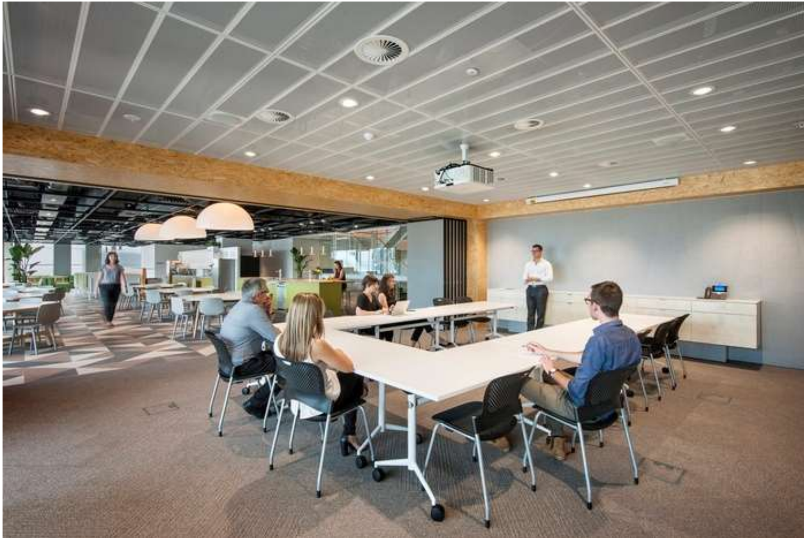
Commercial office with open ceiling (ie no Coanda effect)
