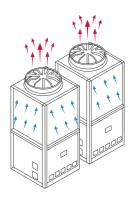
Poor heat transfer at the bottom of coil
