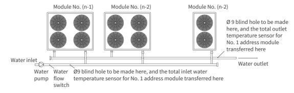
. The unit shall supply the water inlet and outlet temperature sensor, and the user shall arrange them according to the on-site condition. 2. The corresponding water flow switch is not supplied, and shall be provided by the user.
