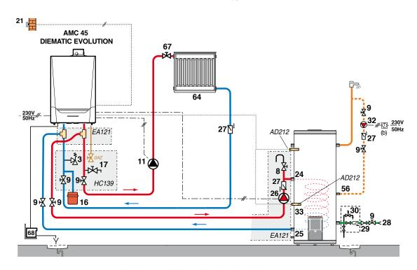
Installation of an AMC DIEMATIC EVOLUTION with 1 direct circuit + 2 circuits with mixing valve + 1 BPB/BLC type domestic hot water tank, all four behind a low-loss header
