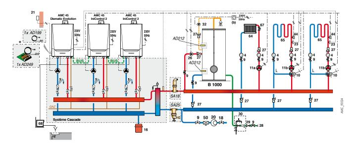
specific case of a cascade installation with more than 2 secondary circuits with mixing valve: installation of 2 AMC PRO...DIEMATIC EVOLUTION boilers in cascade with 4 circuits with mixing valve and one circuit with convection fans. DHW is made by an FWPC instant DHW tank
