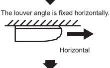
When the discharge temperature is higher than 30°C, the louver angle is automatically returned to the setting condition.
