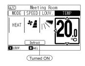
• Operation Stoppage during Defrosting Operation If the unit operation is stopped during defrosting operation, the operation continues with the RUN indicator (Green) turned OFF. The operation stops after defrosting operation.
