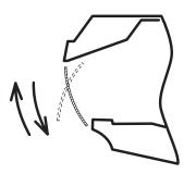
• When "RUN" switch is pressed from the wired controller, the swing louver will be opened automatically. At this time, for cooling, dry and fan operation, the indoor unit is operated with the set temperature after the fan speed "SLOW" operation is performed for approximately 20 seconds.
