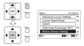
(2) "Motion Sensor Setting" is displayed. The highlighted item is shifted to "Sensor", "If absent" and "Check interval" by pressing "△" or "▽".
