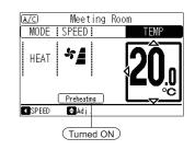
• During Hot Start (for Heating Operation Only) "HOT-START" is turned ON.
