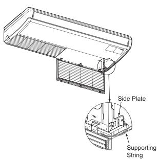
• While the air inlet grille is being opened, depress the knobs of hinge (①), push the air inlet grille toward arrow direction (②) and remove the air inlet grille.
