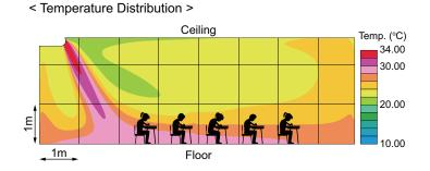
The comfortable heating air reaches every corner of the room, mainly around floor, during the heating operation.
