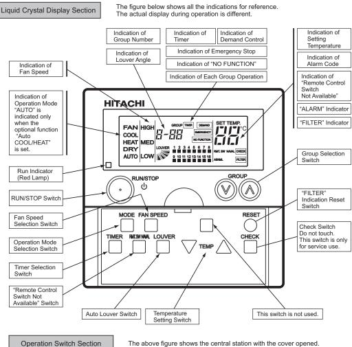
The above figure shows the central station with the cover opened.
