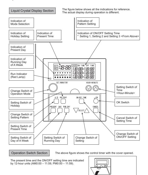
When opening the cover, pull the cover in the direction
