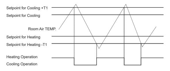
T1: Differential temperature for cooling/heating changeover
