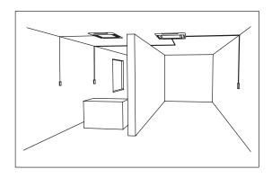
One optional wired controller can start/stop up to 16 indoor units.
